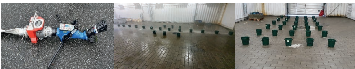
Figure 1: The TFT Blitzfire series water monitor used the tests (left) and the arrangement of the buckets for the 1.0 wide spray (middle) and 3.0 m wide spray (right).
